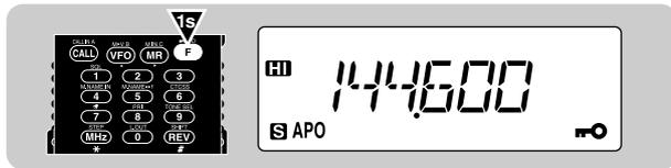
You may want to use the **Tuning** control when in Transceiver Lock mode. Access Menu No. 9 (ENC) to switch the Tuning Control Enable function ON or OFF (default).
